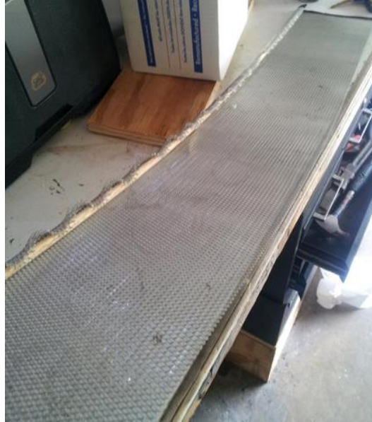
Figure 5: Steel Mesh section of net. Bottom of the net is shown, revealing wooden dowels.
