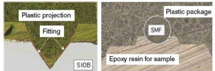
Figure 9 Cross-sections of V-groove alignment on silicon substrate (left) and omega groove of plastic mold (right).
