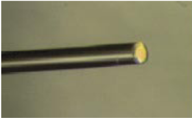
Figure 10 WDM filter vapor-deposited on the facet of angle-polished fiber.
