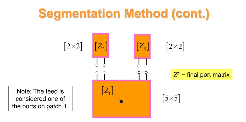
Once the Z matrices of all the patches have been computed, an overall Z matrix of the entire system  $Z^P$  is calculated, by connecting the individual Z matrices and using circuit theory.
