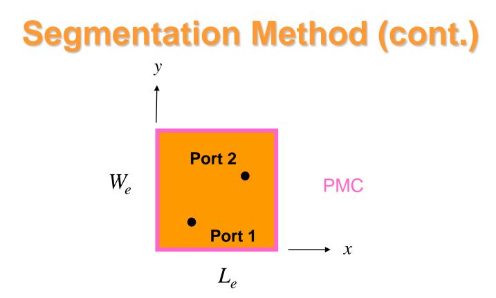
This figure shows a general two-port system for a rectangular patch.
