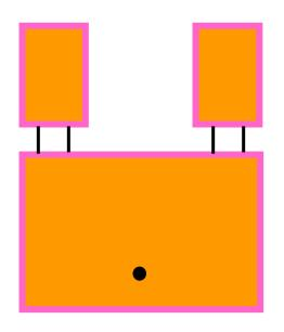
Along the edges where the rectangular patches connect, we introduce ports. The ports connect the patches together.
