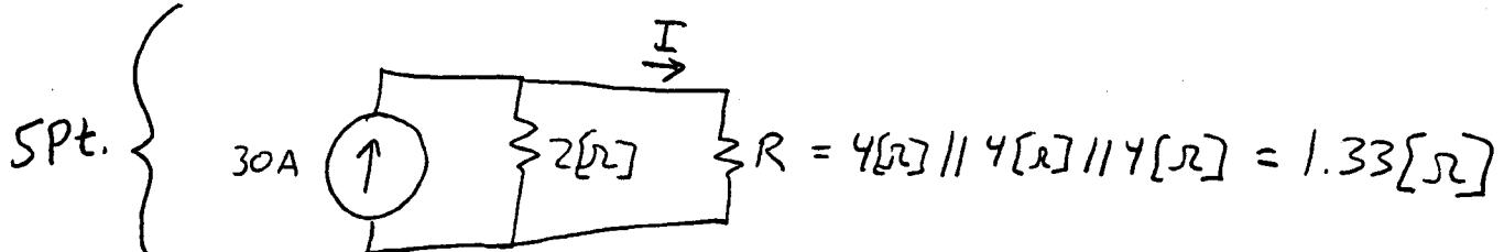
5pt. { Need Power dissipated by  $R$ , heating elements.
