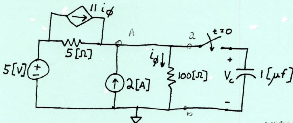
CONVERT CIRCUIT TO THEVENIN EQUIVALENT CIRCUIT WITH RESPECT TO TERMINALS ab
