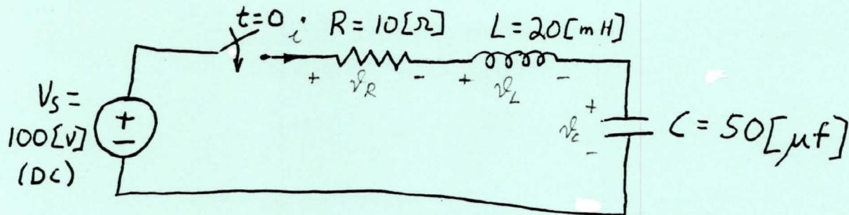
a) Write the circuit integral-differential equation that describes the circuit behavior for  $t \geq 0$ , using current as the variable. Transform it into a second order differential equation.
