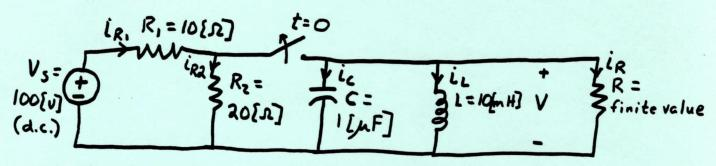
a) Determine the value of  $i_{R1}$ ,  $i_{R2}$ ,  $i_{C}$ ,  $i_{L}$ ,  $i_{R}$ , and v before the switch is opened (t < 0 or t = 0<sup>-</sup>).
