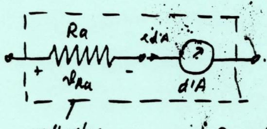
$$v_{RA} = i_{d'A} \cdot R_q = 100 - 0.1 = 99.9 [\text{V}]$$
