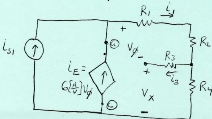
$$i_1 = i_{s1} + i_E = 2\text{[A]} + 6(i_1)(R_1 + R_2)$$
