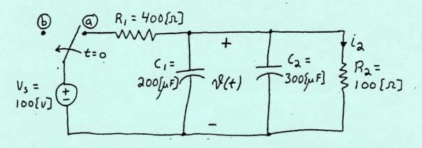
$$\frac{t < 0}{\sqrt{(0^{-})}} = \sqrt{5} \frac{R_2}{R_1 + R_2} = 100 \frac{100}{500} = 20[v]$$
