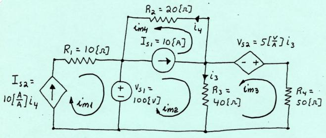
a) Using the number of essential branches and nodes, find the number of independent meshes in this circuit.
