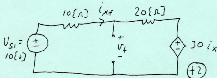
$$\frac{V_{S1} - 30i_x}{30[\Omega]} = i_{xf}$$
