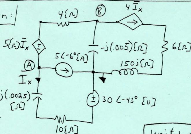
$$\begin{aligned}\bar{Z}_{L_1} &= j\omega L_1 = j50(3) = 150j \Omega \\ \bar{Z}_{C_1} &= \frac{1}{j\omega C_1} = -j(0.005) \Omega \\ \bar{Z}_{C_2} &= \frac{1}{j\omega C_2} = -j(0.0025) \Omega \\ \bar{I}_{S1} &= 5 \angle(84^\circ - 90^\circ) A \\ \bar{I}_{S1} &= 5 \angle -6^\circ A\end{aligned}$$
