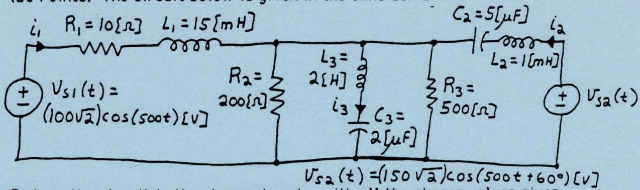
a) Redraw the circuit in the phasor domain, with all the phasor values given as RMS values.
