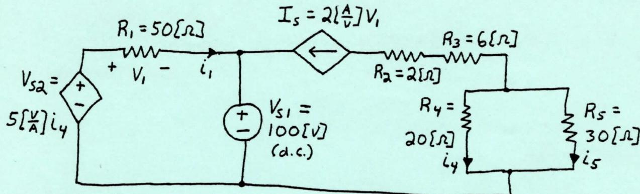
$$(1) \quad i_1 = \frac{V_{S2} - V_{S1}}{R_1} = \frac{V_{S2} - 100}{50}; \quad I_s = 2V_1 = 2 \cdot R_1 \cdot i_1 = 100i_1;$$
