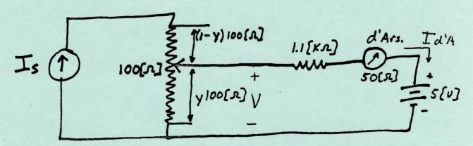
a) A null measurement is obtained when the slide wire is positioned 2/3 of the way up the scale; that is, when y = 2/3. What is  $I_S$  in this case?
