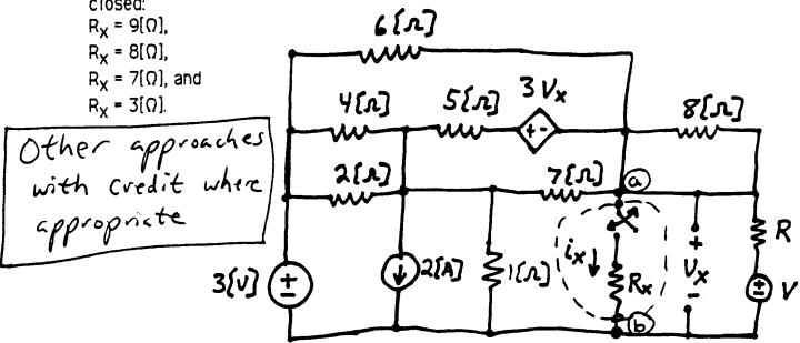
The circuit outside of the dotted line can be replaced by a Thev. equiv. ckt. Using that, we can draw
