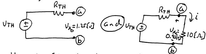
$V_{TH} = 1.25 \{v\} = i = 0.093 \{A\} = 1.25 - 0.93 \{v\}$   $R_{TH} = 3.44 \{x\}$
