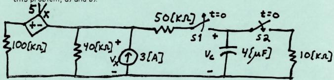
a) Find the Thevenin equivalent with respect to the capacitor terminals for this case. In other words, find the Thevenin equivalent with respect to the capacitor for  $t \le 0$ .
