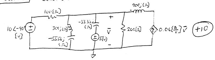
Use complex Node Voltage Method. For V in [Volts]; >>
