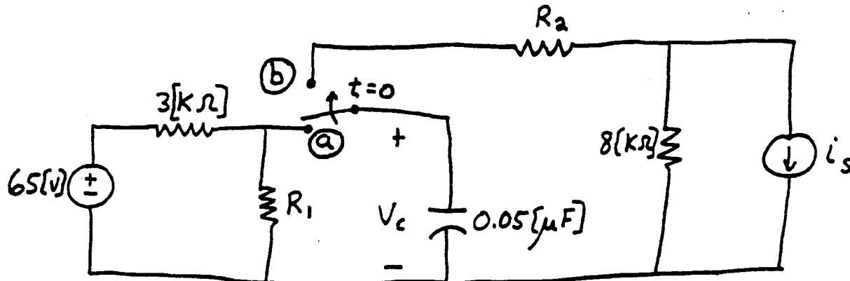
$$v_C(t) = 18 + 17 e^{-t/0.66 \mu\text{sec}} \quad [\text{V}]$$
