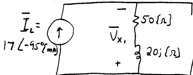
$$\text{+2} \quad \bar{V}_{x_1} = -(17 L -95^\circ) \text{ [mA]} (50 + j 20) \text{ [ohm]}$$
