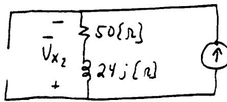
$$\text{+2} \quad \bar{V}_{x_2} = (-6 L -45^\circ) (50 + j 24) \text{ [mV]}$$
