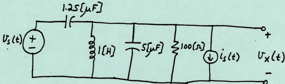
Solution 2 different sources with different frequencies  $\rightarrow$  superposition (+)
