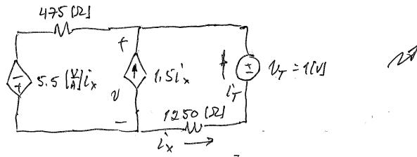
$$\frac{v_{+5.51x}}{475} - 1.52x + \frac{v_{-1}}{1250} = 0$$
