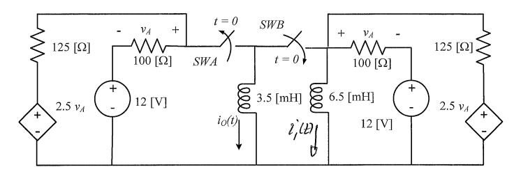
with swA closed and swB open, each inductor is connected to the same circuit, so the initial (txo) current is the same in both, with L >> short for steady state at txo:
