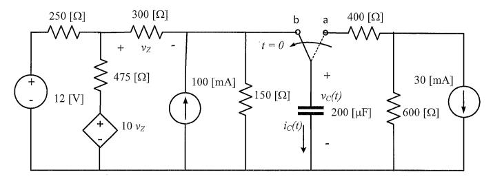
3. {35 Points} The switch in the circuit below was at position 'a' for a long time, and moved to position 'b' at t = 0. At t = 0.1[ms] it moved back to position 'a'. Find  $v_C(t)$  for  $t \ge 0$ .
