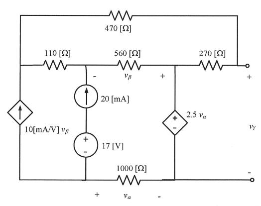
We need to choose two of open-circuit voltage, short-circuit current will corrent, and test source. Since short circuit current will make NB=0, this will simplify things. So will a test source, which removes the branch with the 20[mA] source. These which removes the branch with the 20[mA] source. These two things are the best way to go, but we will do all three.
