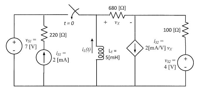
In the circuit shown, the switch was open for a long time, and then closed at t = 0.
