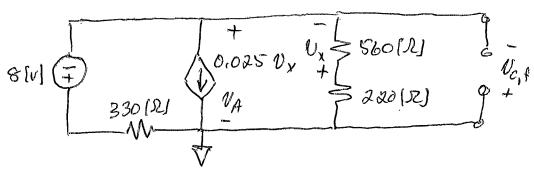
$$\frac{v_{A}+8}{330} + \frac{v_{A}}{560+220} + 0.025 v_{x}$$
