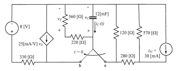
In the circuit shown, the switch was in position 'a' for a long time, and moved to position 'b' at t = 0.
