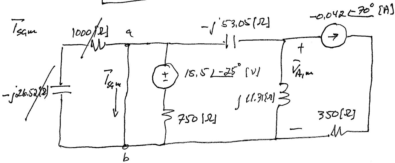
$$\frac{\bar{V}_{A1,m}}{j16.31} - 0.042 \angle -70^\circ + \frac{\bar{V}_{A1,m}}{-j53.05} = 0 \Rightarrow \bar{V}_{A1,m} = 0.6037 [V] \angle 20^\circ$$
