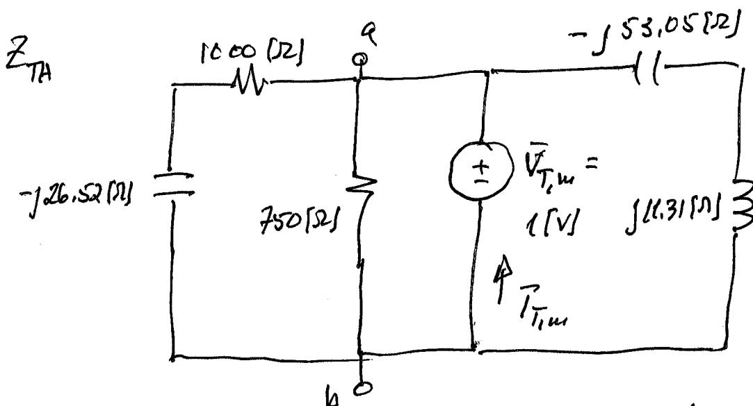
$$\begin{aligned}\bar{T}_{T_{1m}} &= \frac{1}{750} + \frac{1}{-j53.05 + j11.31} + \frac{1}{1000 - j26.52} \\ &= 0.0241 \angle 84.44^\circ \text{ [A]}\end{aligned}$$
