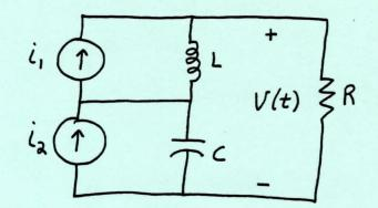
Need to solve using superposition. (w, +wz)
