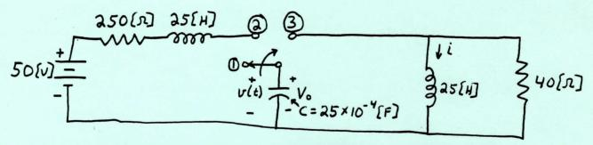
a) At t = 0, the switch is moved to position 2 Determine v(t) after the switch is placed in position 2
