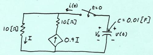
6. (15 Points) In the circuit shown the switch has been closed for a long time. At t=0, the switch is opened. Do not use Laplace techniques to solve this problem.
