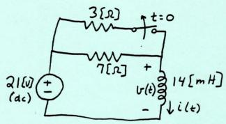
a) Determine the values of i(t) and v(t) for all time after the switch is opened.
