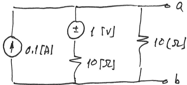
7. Find the equivalent resistance at terminals a, b.
