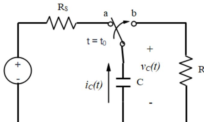
The “natural response” is one in which the capacitor, with a voltage across it, undergoes a switching event that connects it to a resistance only. As for the inductor, that resistance can be a single resistor, or it can be an equivalent resistance that arises from a circuit containing multiple resistors and/or dependent sources.
