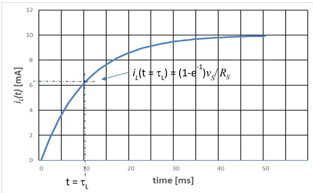
We can now use the current voltage relationship for the inductor to find the voltage across the inductor.
