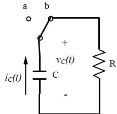
Note that the capacitor current and voltage are in the active sign relationship. You should convince yourself that the signs in this equation are correct. This is a first-order differential equation for  $v_C(t)$ .
