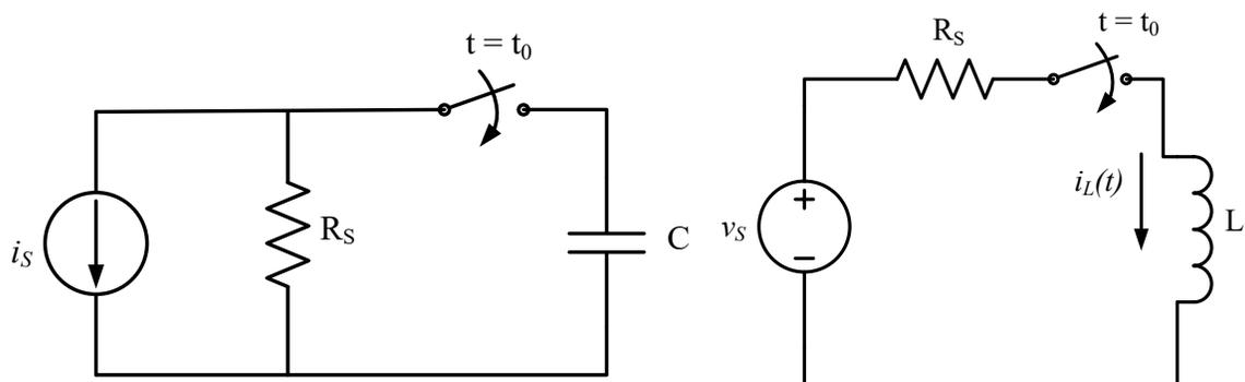
Again, we are using Thevenin and Norton equivalent circuits to represent what gets connected to the inductor and capacitor. Later we will consider more complex circuits.
