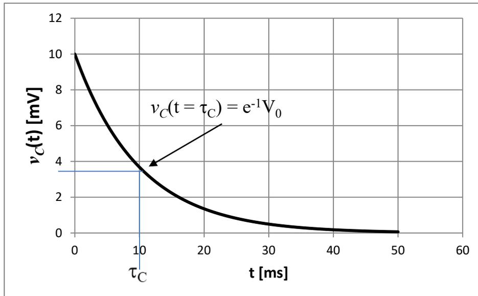
As for the inductor, after five time constants, or  $t = 50$  [ms], the voltage has decayed almost to 0. What is left is less than 1% of the initial value:  $t = 5\tau_C \Rightarrow v_C(t) = 0.0067 v_C(t_0)$ . As we pointed out above, we define a “long time” as five time constants.
