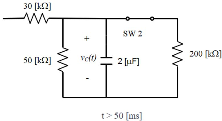
In the last two circuits we could have left the 30 [kΩ] resistor out, but we left it in to make it clear what the circuit configuration is.
