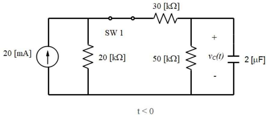
After switch 1 opens, but before switch 2 closes, the capacitor is connected only to the 50 [kΩ] resistor. This is a natural response problem.
