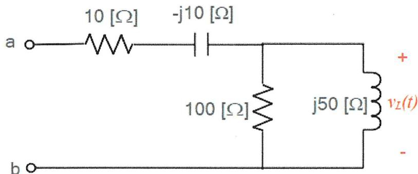
The problem here is that the circuit diagram is clearly a phasor domain diagram, but we have labeled a circuit variable in the time domain. This is an example of mixed domains, and must be avoided at all costs!
