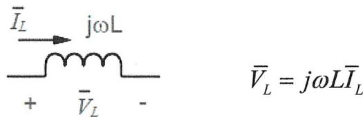
In the phasor domain, we have something that looks like Ohm's Law for an inductor, except that the resistance  $R$  is replaced by  $j\omega L$ . We call  $j\omega L$  the **inductive impedance**. We'll return to the topic of impedance later. Note that because  $j\omega L$  multiplies a current to get a voltage, it must have units of Ohms.
