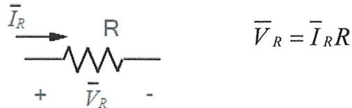
So the phasor transform of the resistor is just Ohm's Law, but with phasors substituted for time domain quantities.
