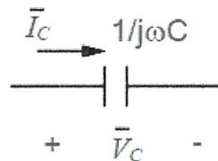
$$\begin{aligned}\bar{I}_c &= -\omega C \bar{V}_c e^{-j90} = j\omega C \bar{V}_c \\ \bar{V}_c &= \left( \frac{1}{j\omega C} \right) \bar{I}_c\end{aligned}$$
