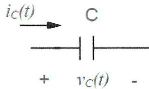
$$\begin{aligned}v_c(t) &= V_m \cos(\omega t + \mathcal{G}) \\i_c(t) &= C \frac{dv_c(t)}{dt} = -CV_m \omega \sin(\omega t + \mathcal{G}) \\&= -CV_m \omega \cos(\omega t + \mathcal{G} - 90^\circ)\end{aligned}$$
