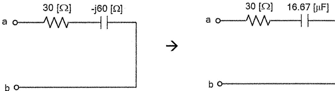
Sometimes it is convenient to work with the reciprocal of the impedance, which is the **admittance**  $Y$ . We then have
