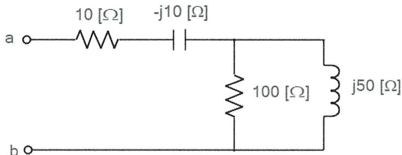
This is the phasor-domain version of the original circuit. We found the capacitive impedance as follows.
