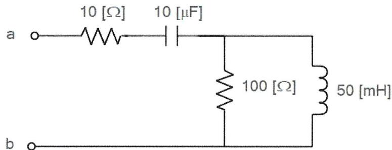
There is no way to combine these circuit elements in the time domain. But if we convert them to the phasor domain, we can add the impedances just as we would resistances. The resistors remain as they are, but the capacitor and the inductor transform to the phasor domain as we have indicated above. To do that, we need the angular frequency  $\omega$ , which we are given.
