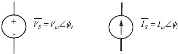
We use the same notation for dependent sources. In this case, the dependent source will depend on a phasor voltage or phasor current.
