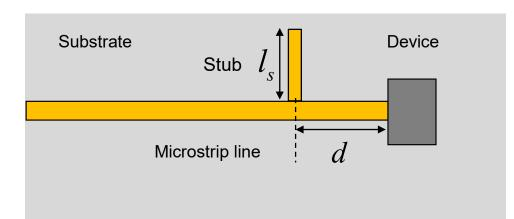
$$SWR = \frac{1 + \left| \Gamma_L \right|}{1 - \left| \Gamma_L \right|}$$
