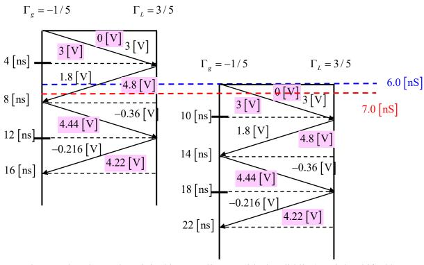
The snapshot due to the original bounce diagram (black solid line) and the shifted bounce diagram (black dashed line) are shown below. The final plot (coming from the black solid plot minus the black dashed plot) is shown in red.
