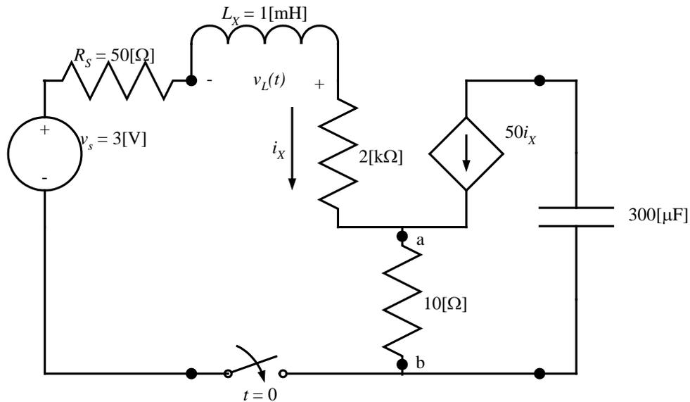
6. For the circuit shown, the switch had been closed for a long time before opening at  $t = 0$ . Find  $i_x(0.4[s])$ .
