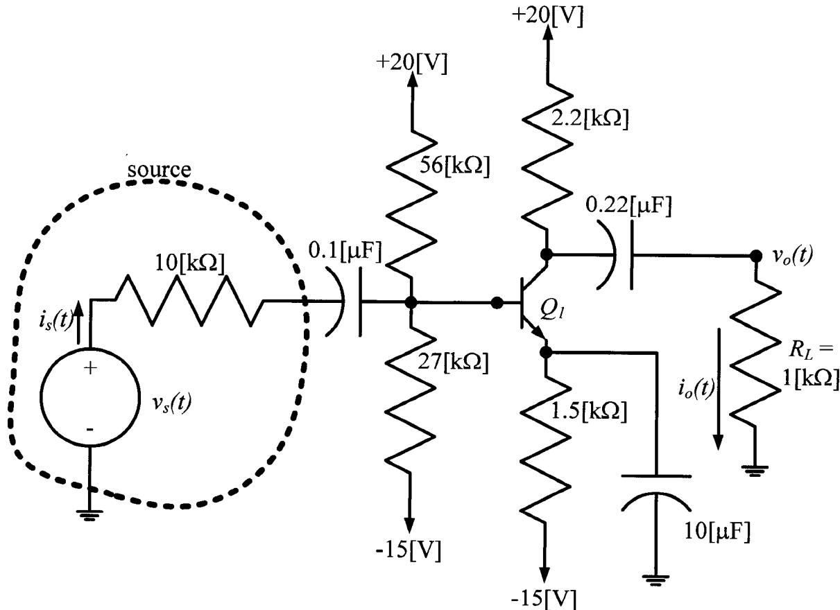
We start with dc analysis. For dc, all capacitors act as an open circuit. Before guessing a region, we choose to find the Thevenin equivalent of the "voltage divider" at the base.
