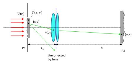
What we can do here is to apply Fresnel diffraction theory twice for each stage:
