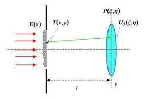
We can apply Fresnel theory as above to find the diffracted field from the object to the plane before the lens. It is:
