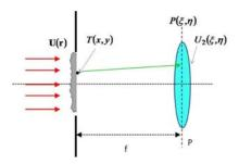
Object right at the front focal plane of lens: what happens at the back focal plane?
