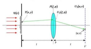
We simply use the result from 1.3 to obtain  $U_2$  and then, Fresnel diffraction to propagate the wave from  $U_2$  to  $U_3$ . From Eq. (1.3.3):
