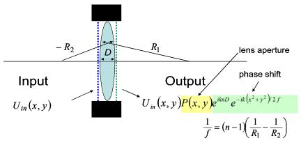
Given an input wave, the output wave can be expressed as:
