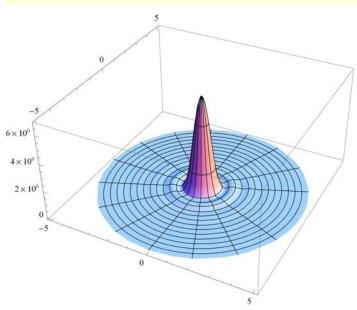
The beam waist diameter  $w = \frac{3.2327 f \lambda}{\pi D} \sim \frac{f \lambda}{D}$  shows that the smaller the lens f-number: f/D, the smaller the waist, i. e. tigher focusing, which indicates the lens optical resolution.
