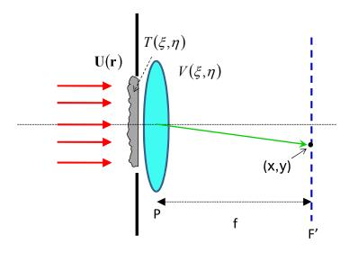
If we neglect the uniform phase term k n D, A beam after thin lens is approximated as:
