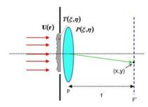
Object right at the front focal plane of lens: what happens immediately after the lens?
