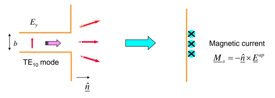
Waveguide with infinite baffle
