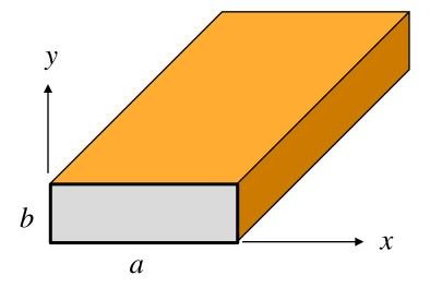
In this example we show that the  $TE_{00}$  mode of the rectangular waveguide is non-physical, since it violates the divergence condition.
