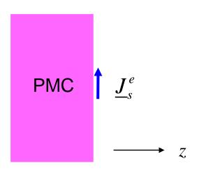
The magnetic current does not radiate on PMC, and is therefore not included.
