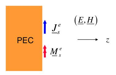
The electric surface current on the PEC does not radiate.
