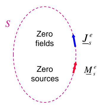
Outside S, these sources radiate the same fields as the original antenna, and produce zero fields inside S.
