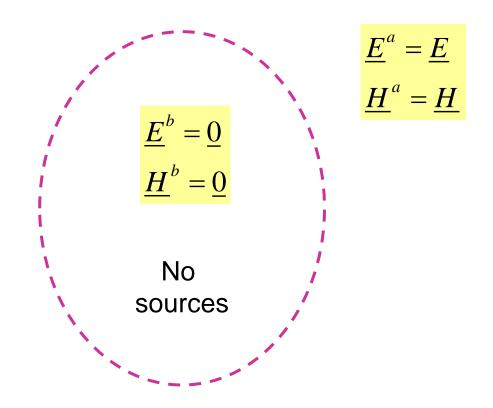
**Note:**  $(\underline{E}^a, \underline{H}^a)$  and  $(\underline{E}^b, \underline{H}^b)$  both satisfy Maxwell's equations.
