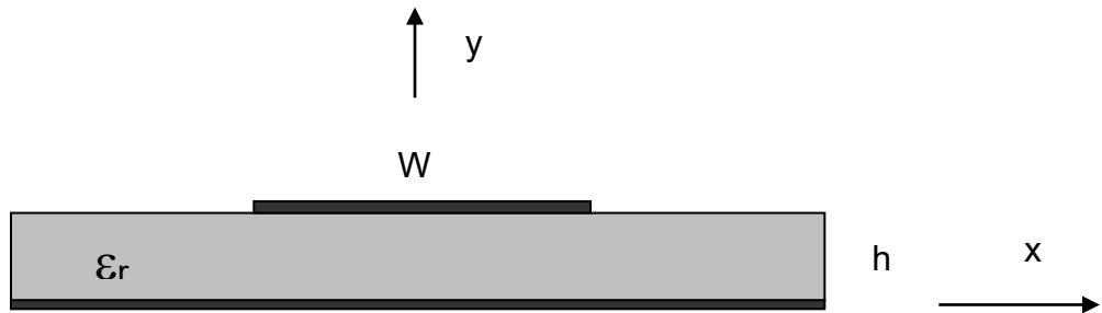
1. Determine the magnetic field in the region under the strip, and the current  $I$  flowing in the  $z$  direction on the strip.
