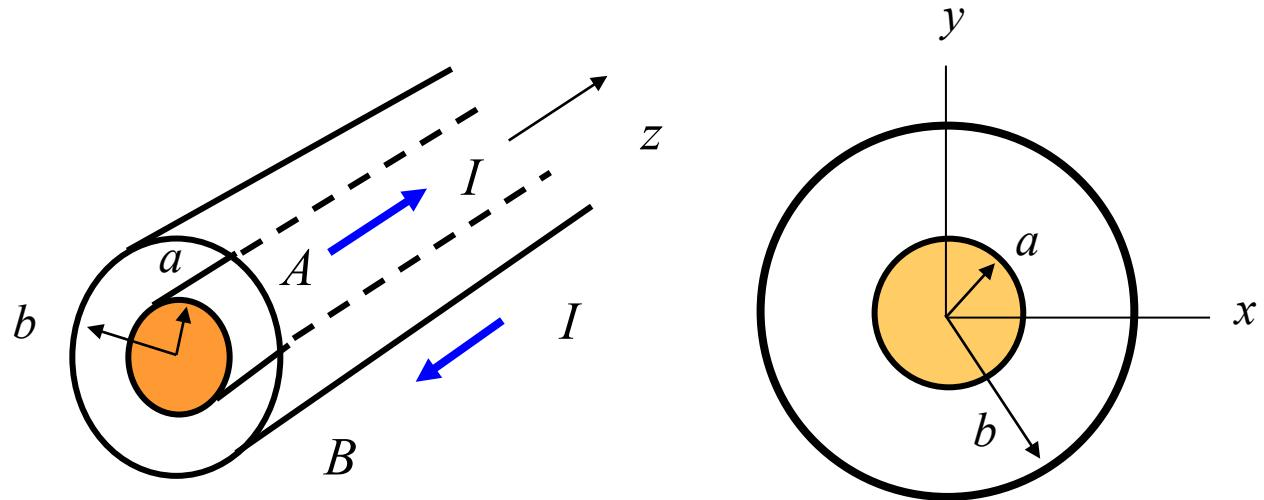
Assume that the electric field of a TEM mode propagating in the  $z$  direction is described in the cross-sectional  $z = 0$  plane by the function
