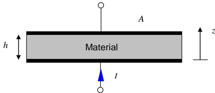
You may assume that the field inside the material is  $z$ -directed, and uniform. The field outside the capacitor may be assumed to be zero.
