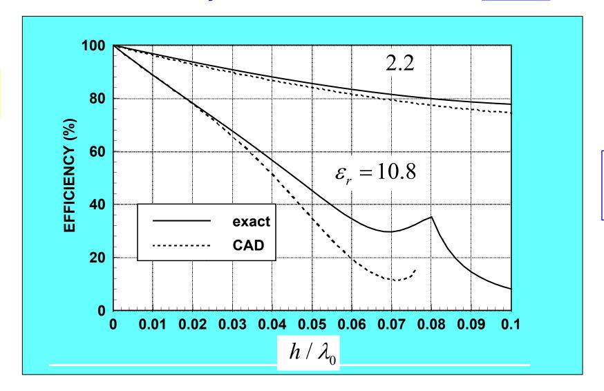
The loss of efficiency here is due only to the surface wave.
