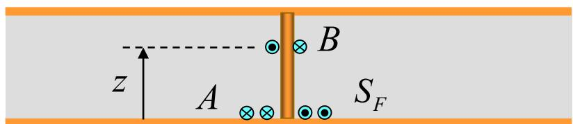
Ampere's law:  $\int_V \underline{H}^a \cdot \underline{M}^b dV = K \int_0^{2\pi} H_\phi^a(a, z) ad\phi = KI(z) = I(z)$
