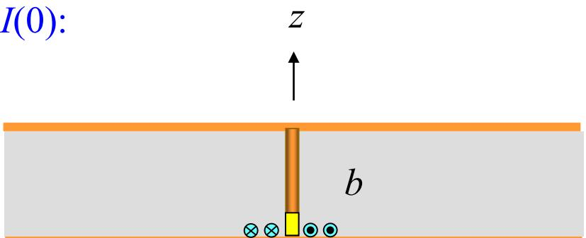
$$I(0) = -\frac{2\pi}{\ln(b/a)} \int_a^b H_\phi^{\text{gap}}(\rho, 0) d\rho$$
