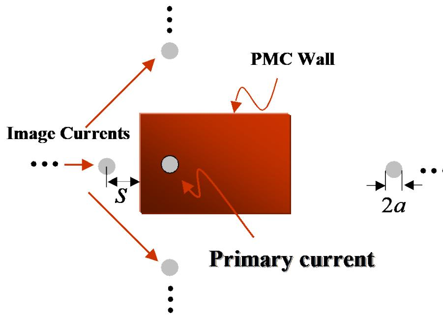
The probe images are reflections of the original probe current about the four PMC walls.
