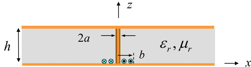
$$Y_{\text{in}} = 1 / Z_{\text{in}} = j \left( \frac{1}{\eta_0} \right) \left( \frac{1}{k_0 h} \right) \left( \frac{1}{\ln(b/a)} \right) 4\pi\epsilon_r \sum_{m=0}^{\infty} \frac{H_0^{(2)}(k_{\rho m} b) - H_0^{(2)}(k_{\rho m} a)}{(\bar{k}_{\rho m}^2)(1 + \delta_{m0}) H_0^{(2)}(k_{\rho m} a)}$$
