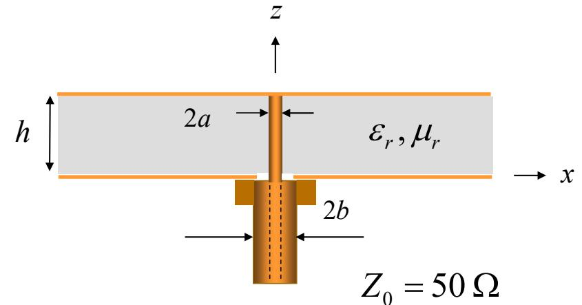
$$\begin{aligned}\varepsilon_r &= 2.2 \\ a &= 0.635 \text{ mm} \\ b &= 2.19 \text{ mm} \\ f &= 2.0 \text{ GHz}\end{aligned}$$
