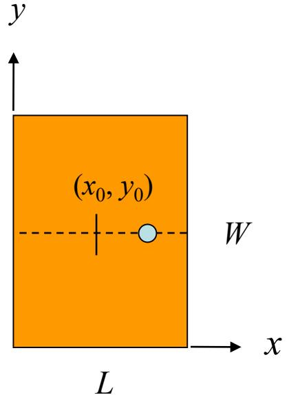
$$\begin{aligned}\varepsilon_r &= 2.2 \\ W/L &= 1.5 \\ h &= 0.020\lambda_0 \\ a &= 0.5 \text{ mm} \\ f &= 5.0 \text{ GHz} \\ Z_0 &= 50\Omega\end{aligned}$$
