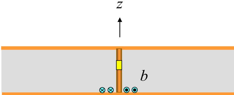
The magnetic current ring  $B$  may be replaced by a 1V gap source of zero height (by the equivalence principle).
